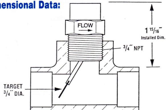
Model 5200 illustrated at no flow condition, red side visible. Unit is installed into a standard PVC 1x1x3/4" SCH 40 reducing tee or a similar method may be used.
